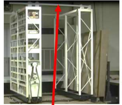
ANTI – TIPPING ROD MECHANISM CONNECTING BODIES ON TOP
